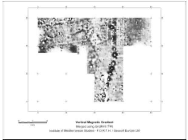
Figure 2. Vertical magnetic gradient grids merged using the GridKnit™ Suturing technique.
