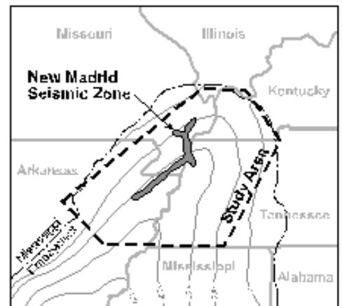
Figure 1. The study area in relation to the Mississippi Embayment and New Madrid Seismic Zone. The poorly consolidated sediments are in excess of 1 km in some parts of the study area.
