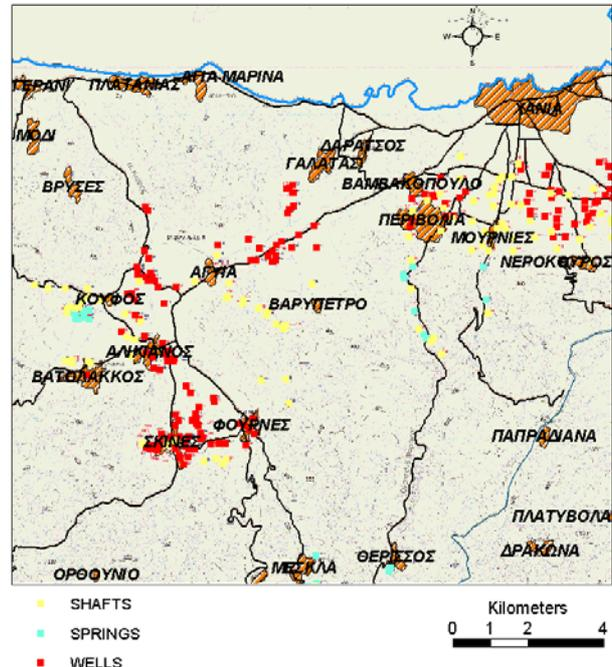
Figure 5. Detail of the digitized locations of wells, springs and shafts as well as the villages and the road network of Chania prefecture, generated from the hydrological maps of Department of Hydrology of the Ministry of Agriculture.
