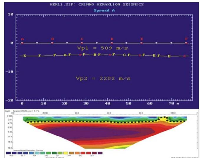
**Fig. 4.** Comparison of the resulted tomographic images from refraction seismics (upper) and geoelectrical tomography (lower) for the same HER11 location.
