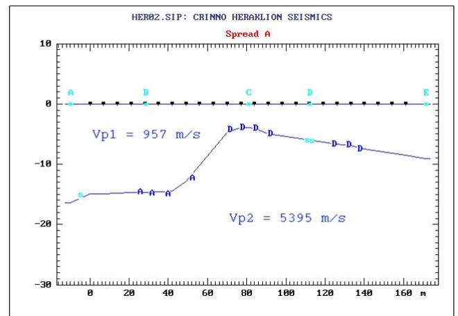
Fig. 3. Resulted geophysical structure for SITE02 in Herakleion city.
